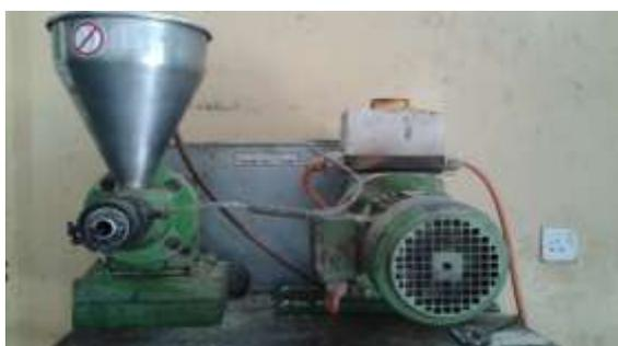
Figure (3-2) Lab scale screw mill used in this study.
