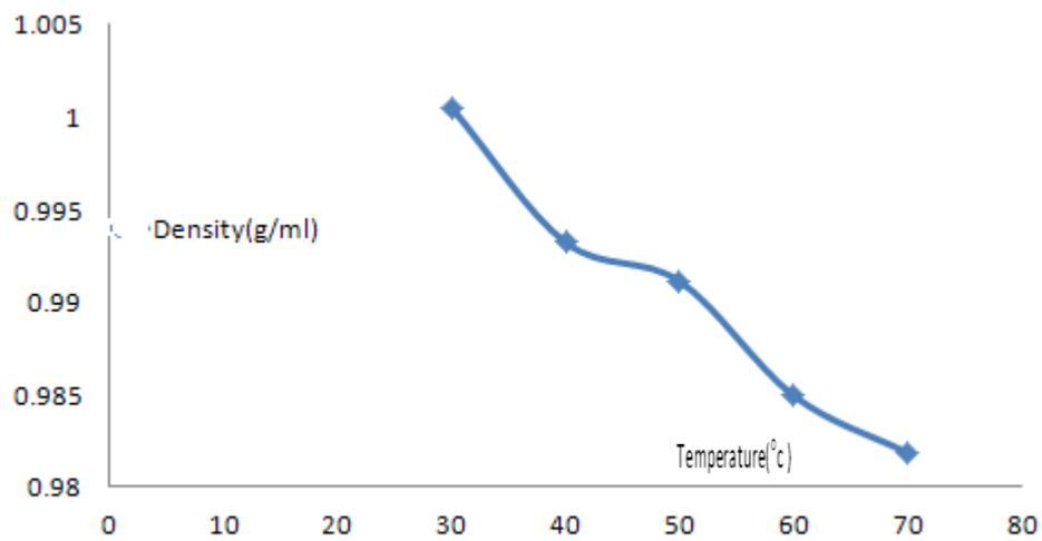
**Fig. (4.3): The effect of temperature on density of (TSS 6%)**
