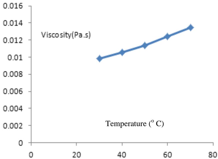
**Fig. (4.2): The effect of temperature on viscosity of (TSS 12%)**
