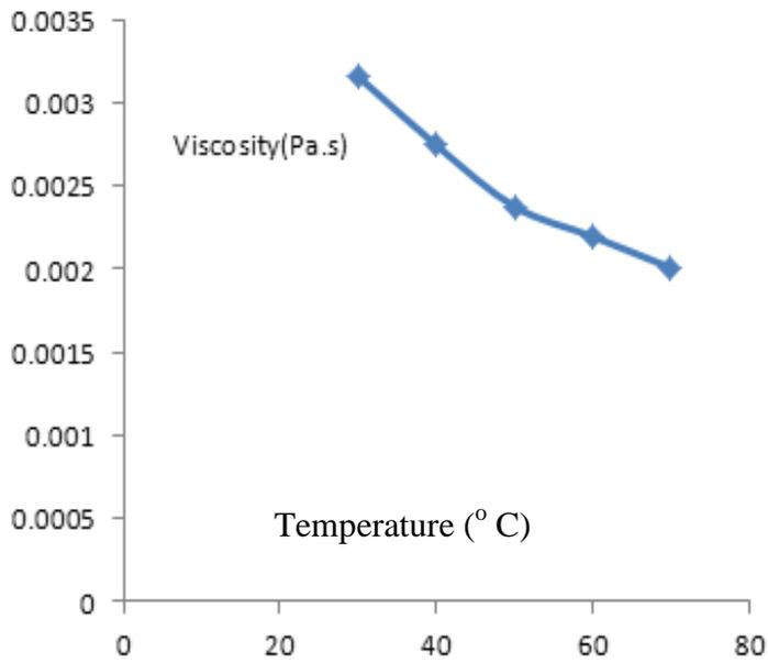
**Fig. (4.1): The effect of temperature on viscosity of (TSS 6%)**
